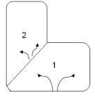
**STEP 3:** Squeegee piece into place working from the middle out, ensuring no tunnels or bubbles have emerged.
